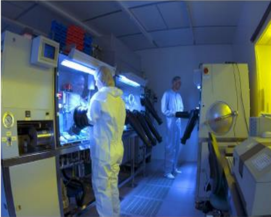
Polymer-Deposition in inert-gas glove boxes by spin coating
